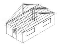
Minimize truss uplift by having the trusses span the width (above left) of the structure rather than its length (above right)
